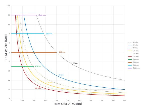
The diagram illustrates that transporting two 70 mm strips requires a Ø80 mm pipe, etc.
